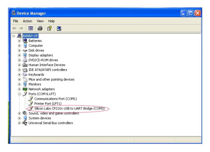
If the COM port does not come up, please check if the USB driver has been probably installed. The USB driver comes with HCS software CD. Make sure the CD has been load to computer first. Then it can program as stand COM port.
