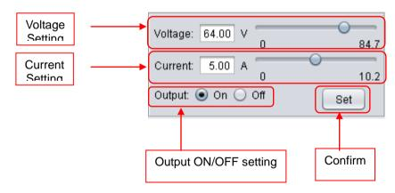
It allow direct input voltage value and current value in setting area or use slide bar to adjust value. After adjust the value, then click set button to confirm setting.
