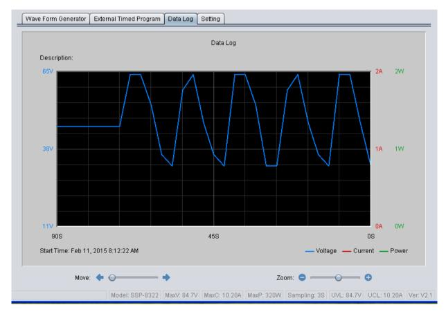
Data log window is used to display output Voltage, Current and Power against time in graphical view.
