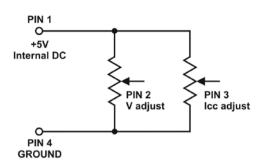
Two variable resistors must be set up at the same time in order for the remote control to be functional.
