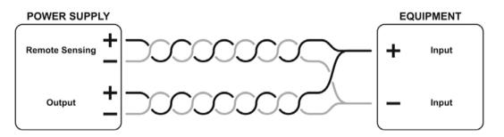
The remote sensing wire should be AT LEAST 22AWG wire size.
